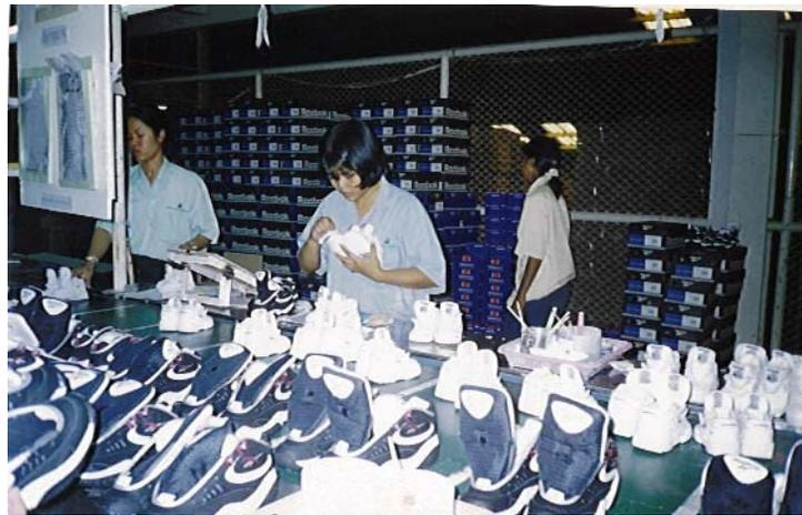
Workers using cleaning solvents without protective gloves. The heat in the factory makes the use of plastic gloves intolerable.
