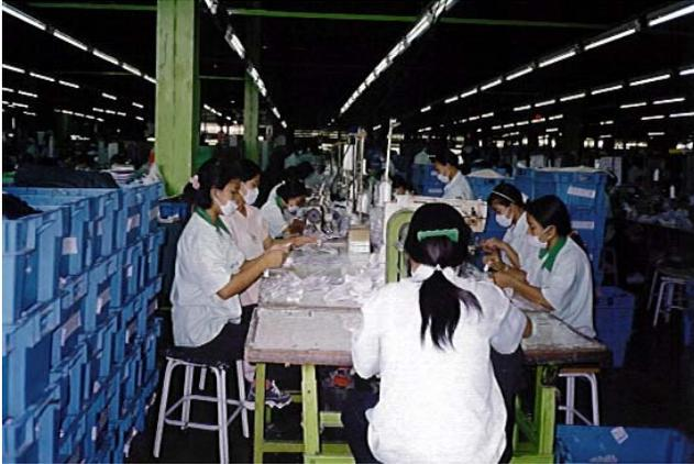
Workers stitching uppers in a Siam Unisole factory. Manufacturers provide cloth-masks to workers to satisfy the codes of conduct. However, as much of the air-born pollutants in the factories are chemical and solvent-based, these masks are of little use.
